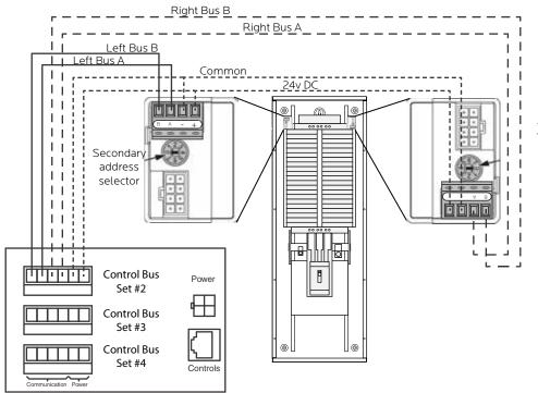
header. Cut two lengths of 18 AWG wire to install jumpers from Left Bus – and + to Right Bus – and +. Right Bus will not operate without these jumpers installed to provide 24VDC power and common.
