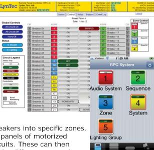
can also allow integrators to set up and divide circuit breakers into specific zones. Consequently, a single controller can operate up to four panels of motorized circuit breakers, which translates to as many as 168 circuits. These can then be easily sub-sectioned into distinct zones and operated by different protocols. For instance, both moving and multicolored lights could be controlled with DMX within a church's sanctuary area while overhead lights could be operated using
