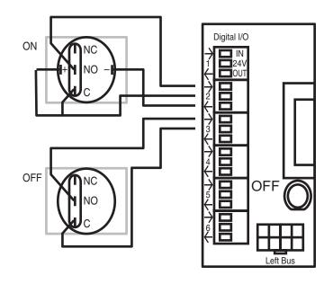
Note: If using emergency override features, fire alarm contact closures must be wired into port 1.
