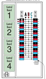
Square D QO342 Load Center Standard back-fed Main Breaker: QO3100VH. 100A, (VH = 22k AIR). Wire: 350 kcmil Al or 250 kcmil Cu. 100% Neutral has one feed lug that accepts one 350 kcmil Al or one 250 kcmil Cu wire.
